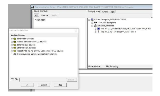
4. When selecting the model do not worry if it is not the exact same model. Example given: You are working with a SLC5/04, but there is no SLC5/04 model with 8K of memory in the Add Device Selection window. Then you will have to choose a SLC5/05 with the same amount memory for it to work.
