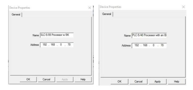
6. Using this configuration, you should be able to communicate with the PLC5 or SLC500 on DH+ from your Panel View
