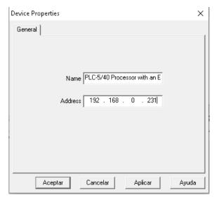
6. Using this configuration, you should be able to communicate with the PLC5 or SLC500 on DH+ from your Panel View
