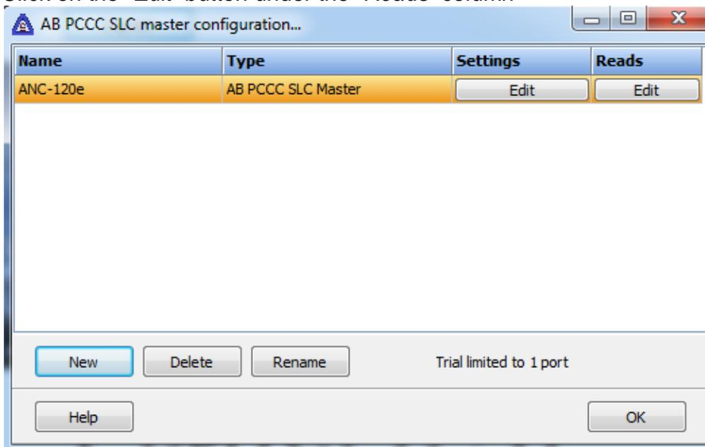
16. Perform a test by configuring one read operation with an address of known value as follows. (In our example we know N7:0 has a value of 1616)
